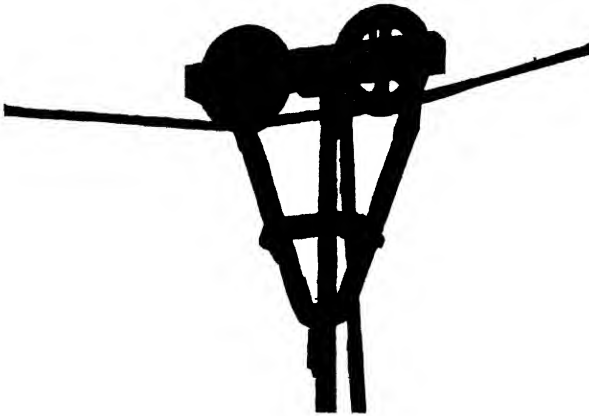
FIG. 18.—Carrier Truck or Runner. Perspective View
